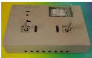
The charger part has two places for batteries. Set the jumpers according to the battery. The 60 mAh must be put on the side. The 20 mAkh can be sqeezed inside. Plantraco designed the box for one single rectangular 90 mAh accumulator that fit inside.
